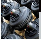
Oil bath axles keep bearings evenly and completely lubricated.
